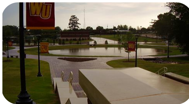
The Campus Green collects water after a storm that would otherwise flood the surrounding sidewalks. Without this design, students would be forced to splash through water after a heavy rain.
